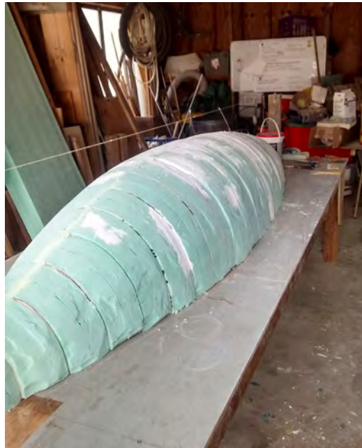
Foam inserted into frame and roughly sanded (March 6).
