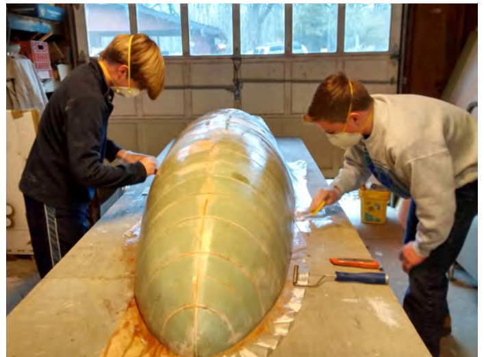
Daniel and Sean apply the "veiling layer" of fiberglass on the plug (March 13).
