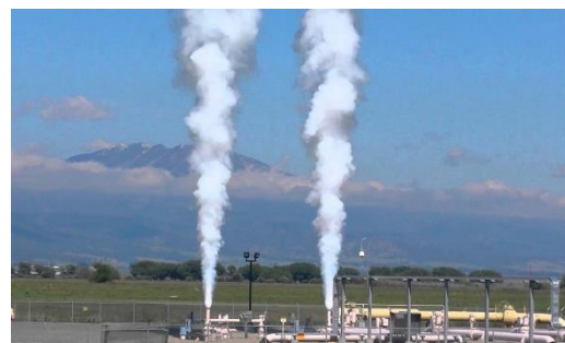
Figure 2 Example of a blowdown in Oregon, from https://www.youtube.com/watch?v=WtSH5V1YQvQ . YouTube has numerous examples. Plume visibility is due to condensation caused by the rapid expansion of the pressurized methane.
